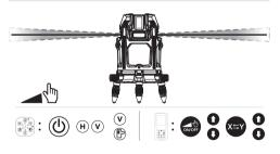
• Activate the manual slope mode by pressing the manual slope button **[n]** on the remote control. You can also activate the slope mode by holding down the power button **[A]** of the device for approx. 2 sec. until a small beep sounds. By releasing the power button **[A]** the slope mode becomes active.
