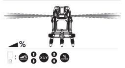
• Activate the digital slope by pressing the digital slope button **[o]**.
