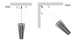
Press the button to stop continuous measurement. The values for maximum and minimum distances are shown in the display as well as the last measured value in the summary line.
