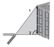
• Indirect measurement - determing a distance using 2 auxilliary measurements e.g. for measuring building heights or widths. It is helpful to use a tripod when measuring heights that require the measurement of two of three measurements.
