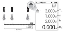
If the distance  $T_n$  to the nearest target point is in front of you, an upward arrow will appear on the left side of the screen. The distance  $D_T$  will be displayed as a positive value in the Main data line [A].
