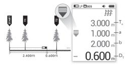
If the distance  $T_n$  to the nearest target point (based on the current position) is behind you, a downward arrow will appear on the left side of the screen. The distance  $D_T$  to this point will be displayed as a negative value in the Main data line [A].
